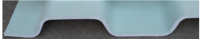
Closeup view of test specimen material showing face, edge and corrugated profile
