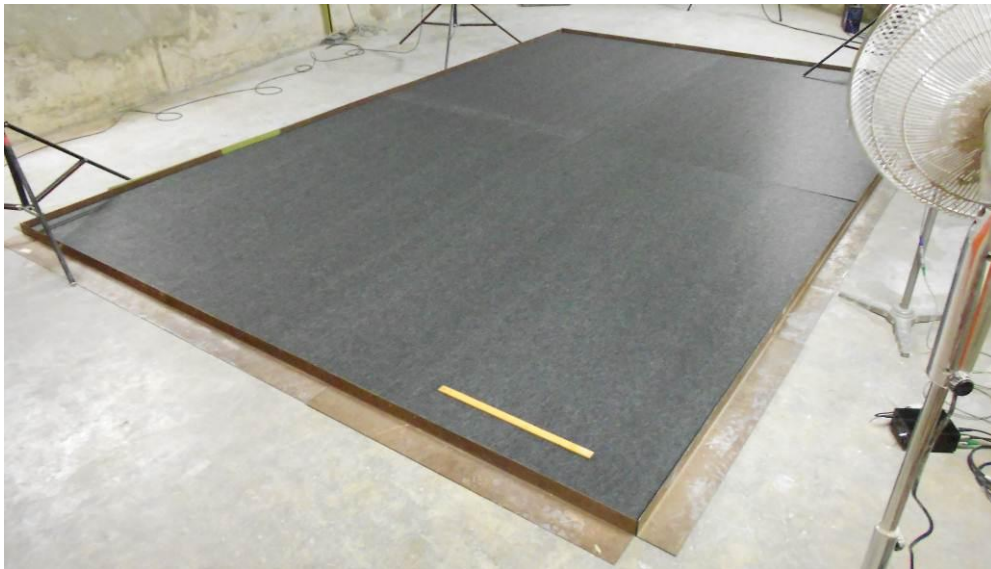
Figure 2: Echo Panel 24mm tested with no air gap installed in Reverberation Chamber
