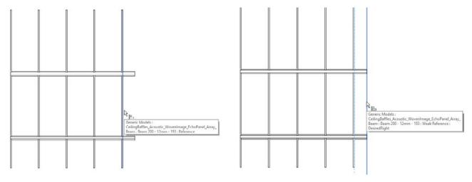
Please note that there may be a necessity to retain the overhanging rails in the situation where a negative detail/shadow line arrangement is desired by combining multiple instances of baffles (see Section 3.4.3).
