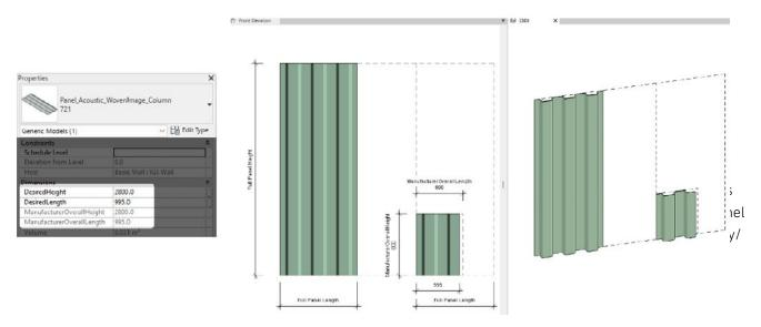
The provided **DesiredHeight** and **DesiredLength** parameters can be updated to resize the panel. The values entered for these parameters are validated against the **ManufacturerOverallHeight** and **ManufacturerOverallLength** to ensure that a full single panel size is not exceeded, and that panels can only be cut on a flat surface, as shown in the image below.
