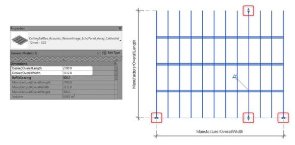
Overhanging rail ends can be adjusted to terminate at the outside face of the final baffle by using the align tool (AL) in a plan or side view. With the align tool active, first select the outermost face of the final baffle in the sequence as the alignment reference, then use the TAB key with the mouse hovering over the overhanging rail ends to select the 'DesiredRight' reference before clicking to apply the align command.
