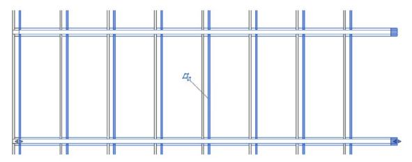
Ensure that the 'ShowCrossrails' parameter is deactivated on this copied instance to avoid duplicate rails and cables. It is important that the installation methods and suspension lengths (if applicable) are identical across all instances used within this configuration to guarantee correct horizontal alignment. Rail ends can be adjusted to suit as per the steps outlined in Section 3.4.1.
