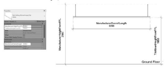
The calculated **TileMountHeightFromFFL** within the Fuji rail family allows for easy vertical alignment of standalone Fuji tiles to the rail's underside. The **ManufacturerHeightFromFFL** of the Fuji tiles should be updated to match the **TileMountHeightFromFFL** value of the supporting rail.
