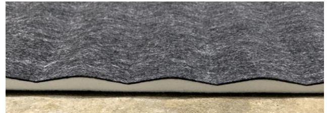
Side view of panel tested including sound-incident embossed surface.
