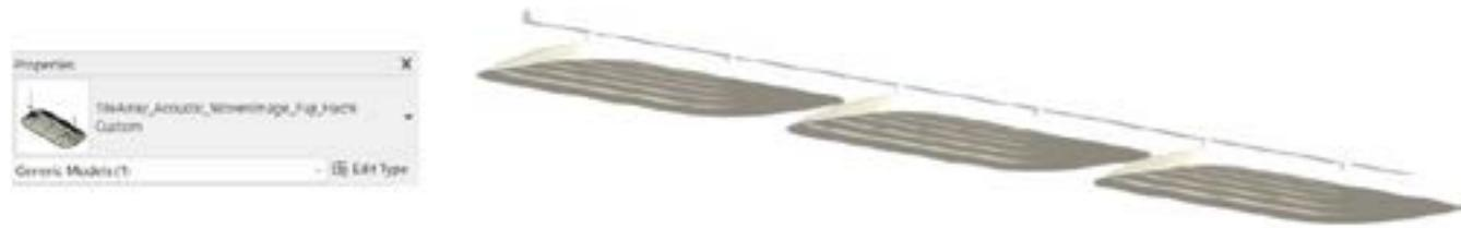
Select this newly placed Custom Fuji system/tile and access the Edit Type dialogue (1). From here, duplicate the type (2) and rename to feature the desired colour(s) to be applied to the tile (3). Once the type has been duplicated, update the **TileTopMaterial** and **TileBottomMaterial** parameters with the appropriate fabric colour materials available within the Woven Image Virtual Showroom file (4). Select OK to apply all changes and reveal the custom Fuji tile solution (5).
