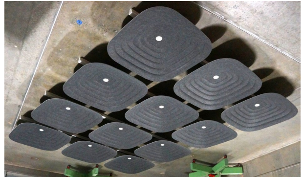
Specimen as tested (image inverted to depict ceiling installation)
