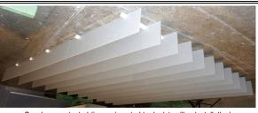
Specimen as tested (image inverted to depict ceiling installation)
