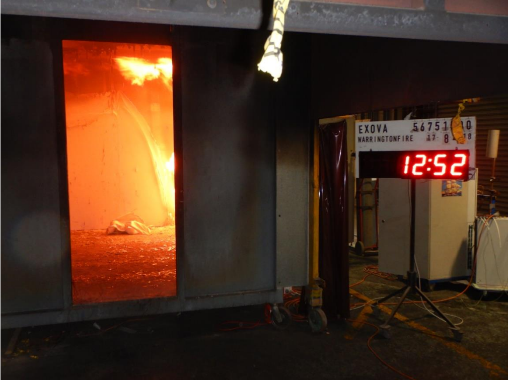
Figure A4.5 Specimen 12 minutes 52 seconds after commencement of the reaction to fire test.
