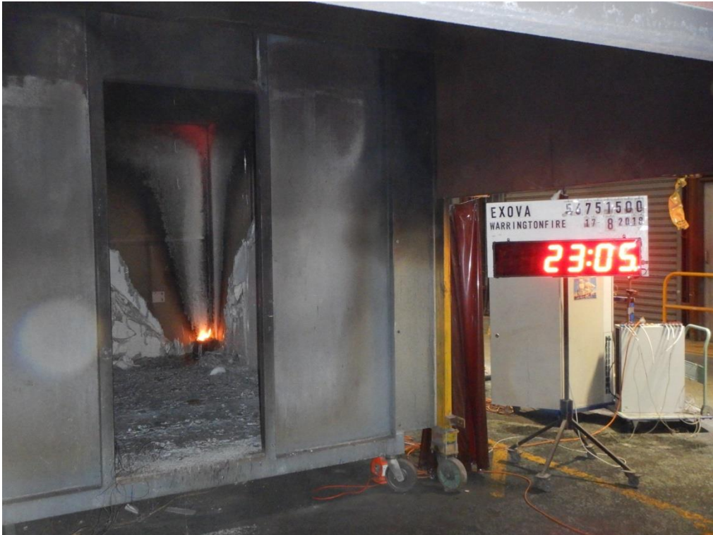
Figure A4.8 Specimen 5 seconds after burner cut off
