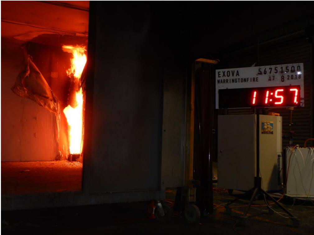
Figure A4.4 Specimen 11 minutes and 57 seconds after commencement of the reaction to fire test.
