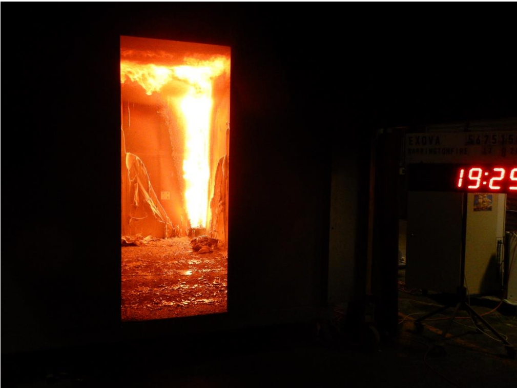
Figure A4.6 Specimen 19 minutes 29 seconds after commencement of the reaction to fire test.
