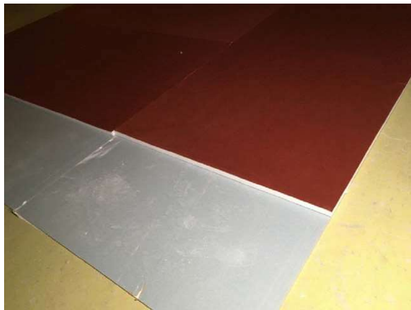
Figure 1: 10mm plasterboard on chamber floor
