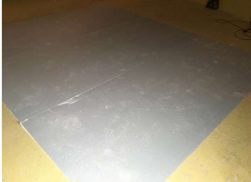
Figure 1: 10mm plasterboard on chamber floor
