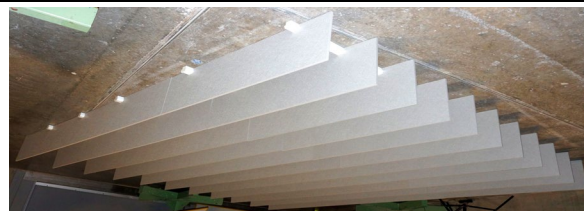
Specimen as tested (image inverted to depict ceiling installation)
