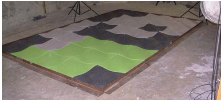
Figure 2: “3D Tile-Dune” tile tested with no air gap installed in Reverberation Chamber
