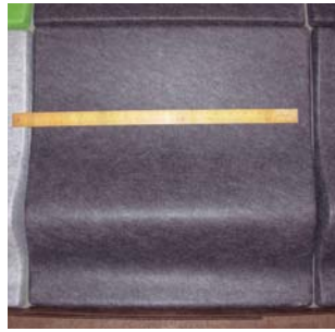
Figure 2: “3D Tile-Wave” tile tested with no air gap installed in Reverberation Chamber
