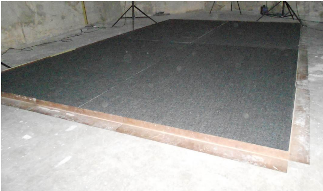
Figure 2: Echo Panel 24mm tested with a 20mm air gap installed in Reverberation Chamber
