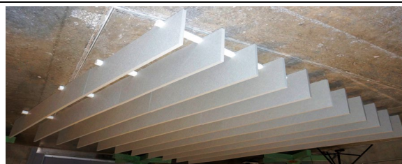
Specimen as tested (image inverted to depict ceiling installation)
