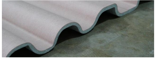
Closeup view of test specimen material showing face, edge and corrugated profile
