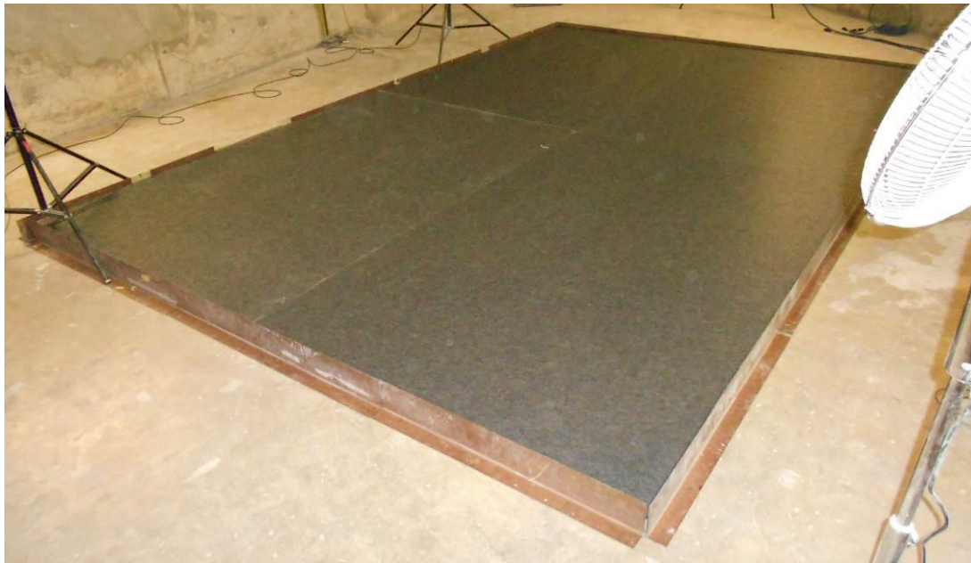
Figure 2: Echo Panel 24mm tested with a 50mm air gap installed in Reverberation Chamber
