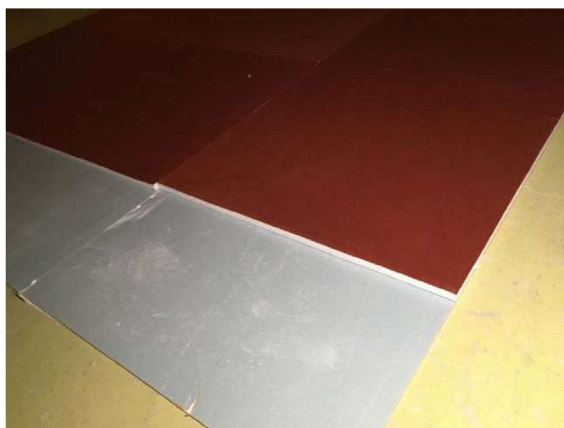
Figure 1: 10mm plasterboard on chamber floor
