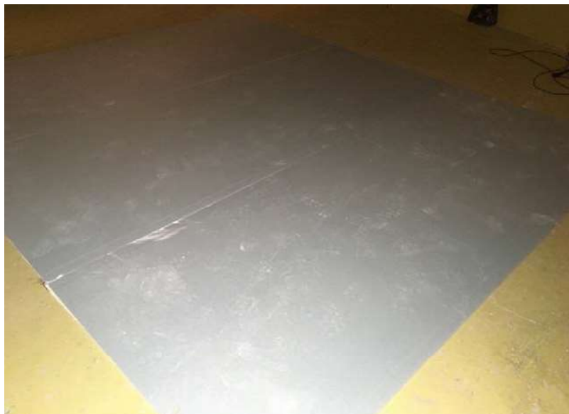
Figure 1: 10mm plasterboard on chamber floor
