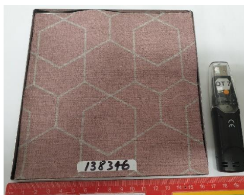
Focus Print – Woven Fabric with knitted scrim and surface print 100% Polyester, 380 g/m 2
